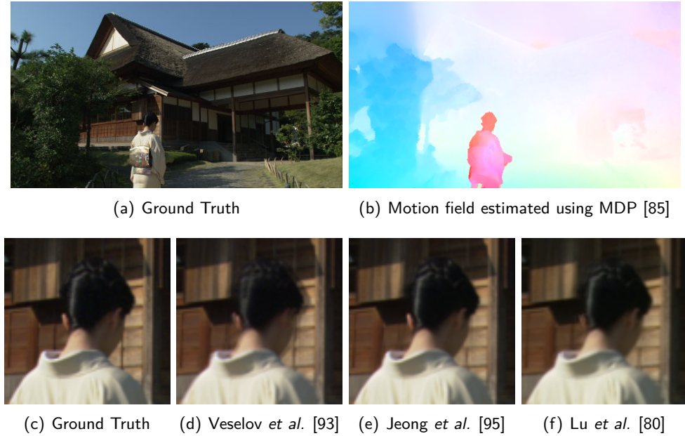
Figure 3.5: Example interpolated frames from the “Kimono” sequence, obtained using different TFI schemes. (a) shows the original frame; (b) shows the motion, estimated using MDP-flow [85]; the second row shows crops of (c) the ground truth, (d) the interpolated frame using a target-anchored scheme [93] without occlusion handling, as well as reference-anchored schemes with (e) implicit [95] and (f) explicit [80] occlusion handling.
