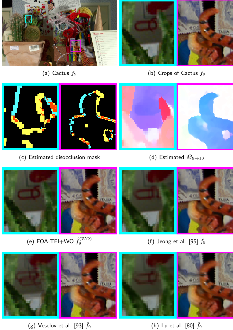
Figure 6.16: TFI comparison on "Cactus" sequence. The first shows the ground truth frame (a), as well as crops of the ground truth frame (b); (c) shows the estimated forward and reverse disocclusion masks (cyan and yellow, respectively), and (d) shows the (colour-coded) mapped forward motion field \hat{M}_{b \rightarrow c} . (e-h) show crops of the proposed FOA-TFI+WO (with both texture optimizations), Jeong et al. [95], Veselov et al. [93], and Lu et al. [80], respectively.
