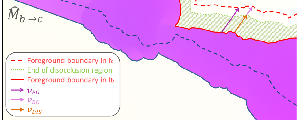
Figure 6.8: The inferred motion field \hat{M}_{b \rightarrow c} is used to identify regions in f_b that are not visible in f_c ; we refer to such regions as “reverse disocclusions”. The start of disoccluded regions is outlined by regions of large negative divergence in \hat{D}_{b \rightarrow c} ; these belong to the trailing side of the foreground object as it moves (in reverse time) from f_c to f_b . \mathbf{v}_{DIS} , which points to the end of the disoccluded region, is defined by the relative difference in motion between the foreground ( \mathbf{v}_{FG} ) and background motion ( \mathbf{v}_{BG} ).
