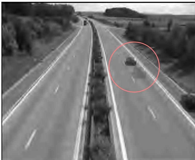
(a) JSIV with the hierarchical arrangement. The average bit rate for the whole sequence is 94.66 kbit/s, the PSNR for this frame is 29.57 dB. The red circle encircles some artefacts.
