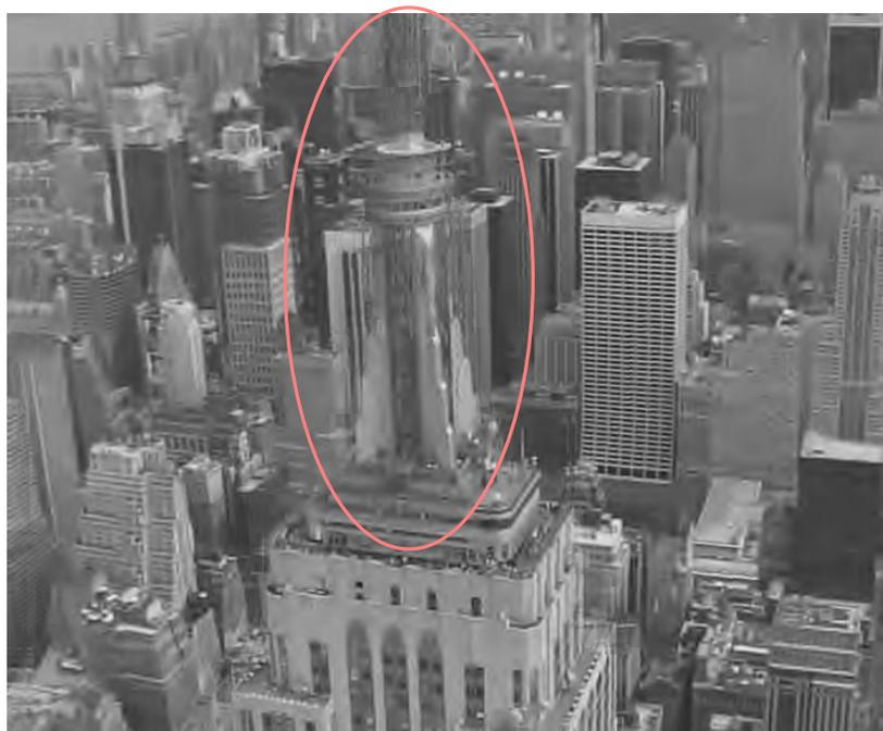
(a) JSIV-H. The average bit rate for the whole sequence is 0.551 Mbit/s, the PSNR for this frame is 28.45 dB. The red ellipse encircles some artefacts.
